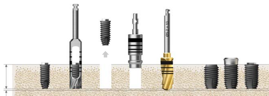
Ø 4.0 Failed Fixture | Ø 4.2/Ø 5.0 Trephine Drill | Ø 5.5 Trial Pin | Ø 4.6/Ø 5.5 Direct Drill | 6.0 Ultra-Wide Fixture
