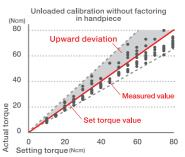
**SM3** calibration ensures outstanding safety because it minimizes deviations and ensures virtually no upward variations from pre-set values. As the graphs show, no calibration can be accurate without taking handpiece usage conditions into consideration.
